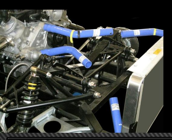
Main chassis rails extend to full vehicle width for greater driver / passenger protection.
