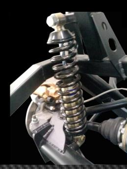
"GAZ gas-filled coil-over damper assemblies with full adjustment for height and damping".
